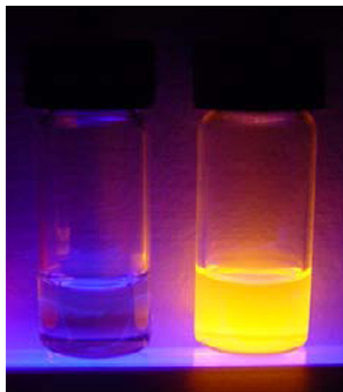
Fig. 4. Bright yellow emission from CdS:Mn/ZnS QDs (right) and deionized water (left) as control. Reprinted by permission from (Ref. [28]), Copyright (2005) American Chemical Society.
